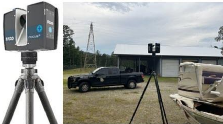
Figure 6: FARO equipment scanning crashed vessel.
