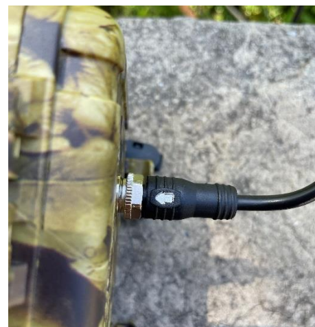
Silver arrow on microphone cable end showing proper orientation of cable inserted into the Anabat unit with silver ring tightened.
