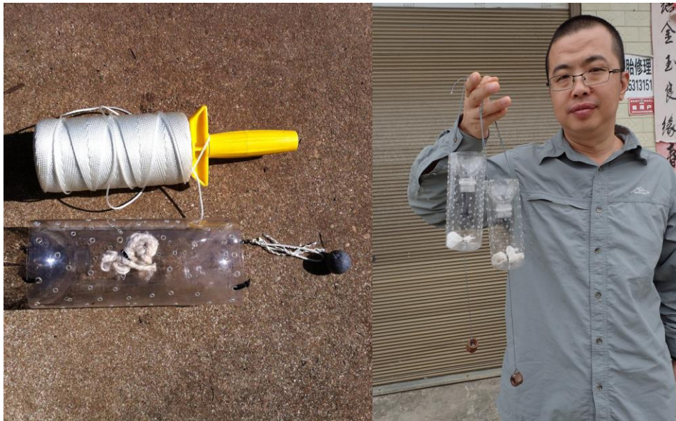
Figure 3. Both single (to the right) and double opening (to the left) well-pipe traps used in this study. Traps are weighted with fishing weights or large steel nuts to orient the traps properly for extraction from a well. Photographs by Dante B. Fenolio.
