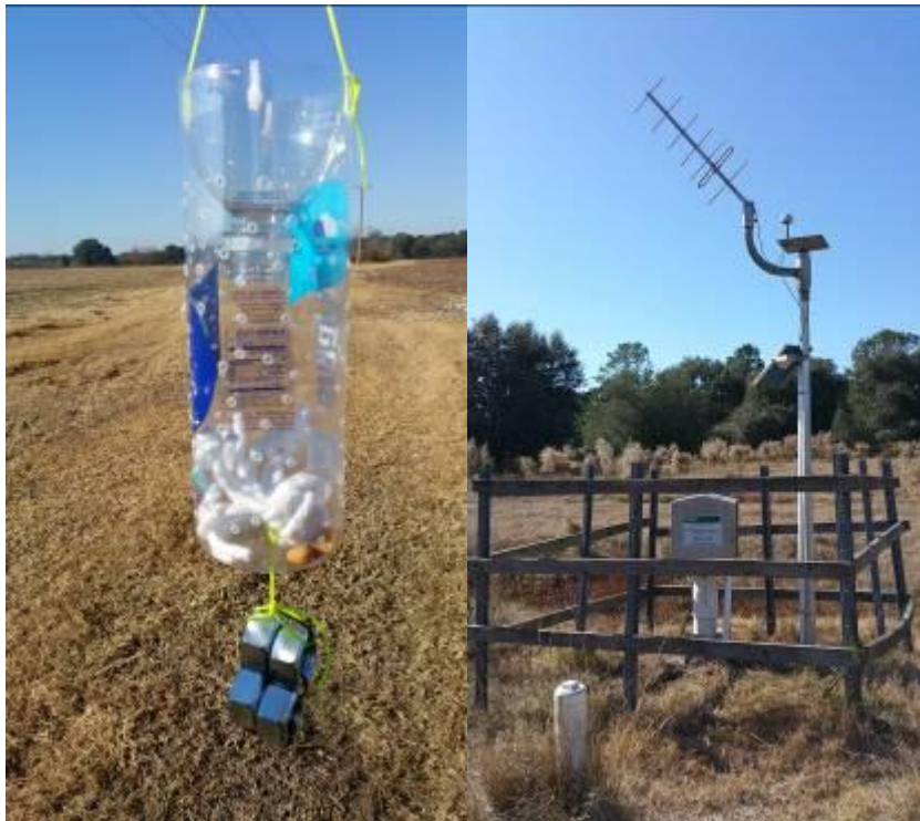
Figure 4. A well-pipe trap ready to be deployed (left) at a USGS groundwater monitoring well (08K001) in Early Co., Georgia (right). Mop head served as refugia for trapped individuals and cashews were used as bait at the bottom of the trap.
