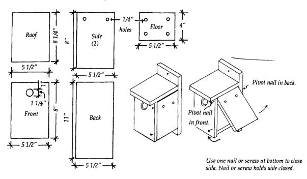
Two "pivot" nails allow side to swing out for cleaning.
