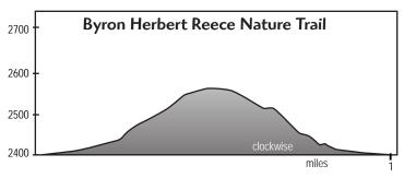
0.8 Mile Partial Loop Average Travel Time: 1 Hour Foot Travel Only Compacted Natural Soil Surface Average Grade: 10%; Max: 20%/150LF Minimum Width: 18 Inches Avg. Cross-slope: 10%; Max: 20%/50LF
