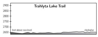
Foot Travel Only Compacted Natural Soil Surface Avg. Grade: 4%; Max: 10%/200LF Min. Width: 30 Inches Avg. Cross-slope: 10%; Max: 15%/30LF Steps on East Side Road is Accessible
