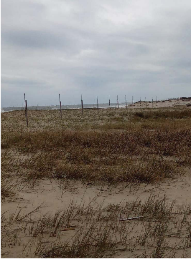
The Rx array currently at Buxton, NC. It is a 12-antenna standard WERA system like the 11-antenna one proposed at Jekyll. The antennas are 10m apart totaling in a 110m array length.
