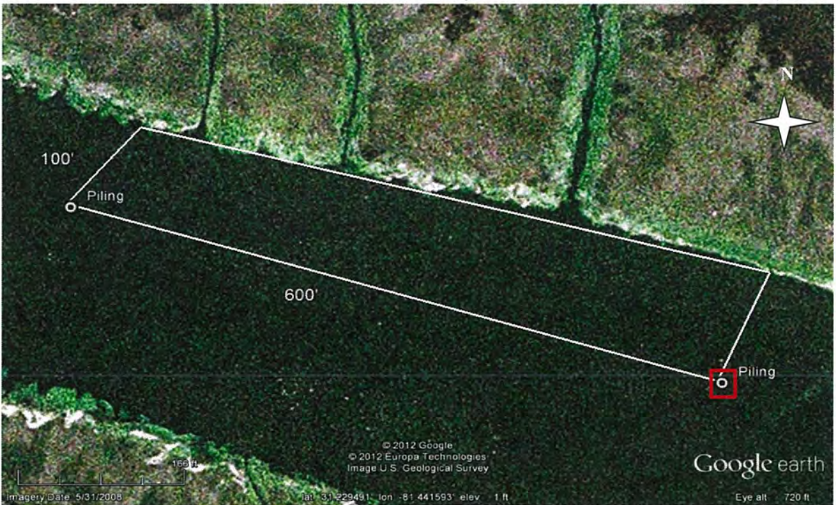
Figure 2. Reef Site Aerial Photograph shown with existing pilings, materials, and footprint (600' x 100'). For navigational purposes the southernmost piling is outlined in red.
