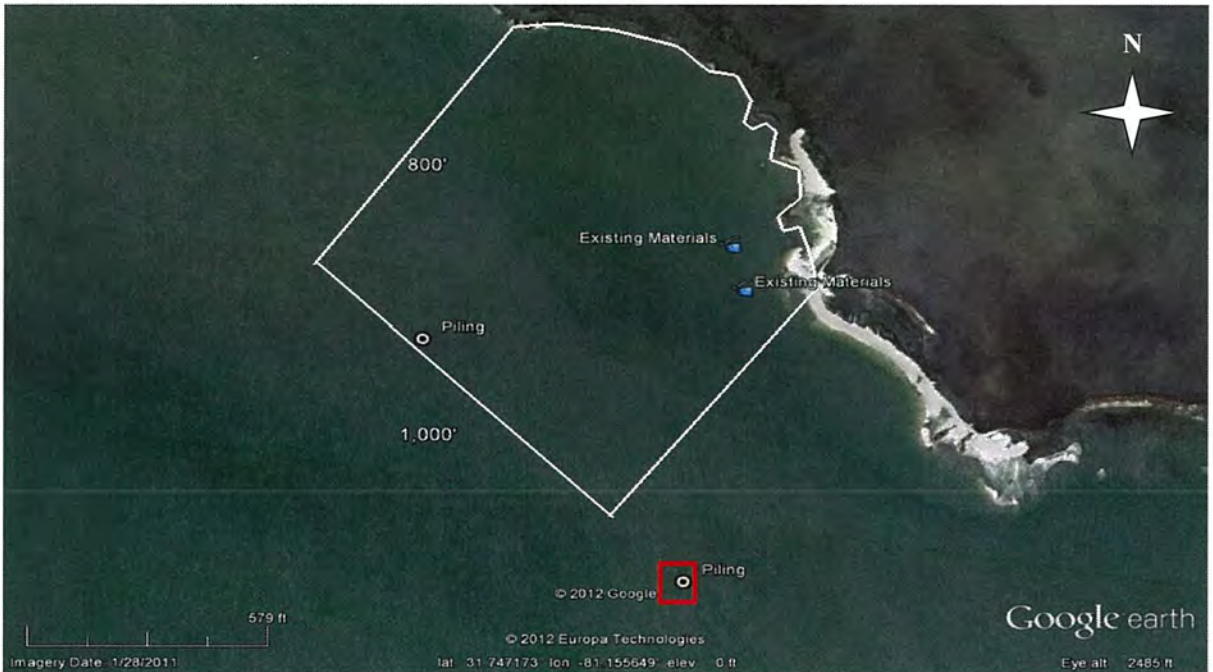
Figure 2. Reef Site Aerial Photograph shown with existing pilings, materials, and footprint (1,000' x 800'). For navigational purposes the southernmost piling is outlined in red.
