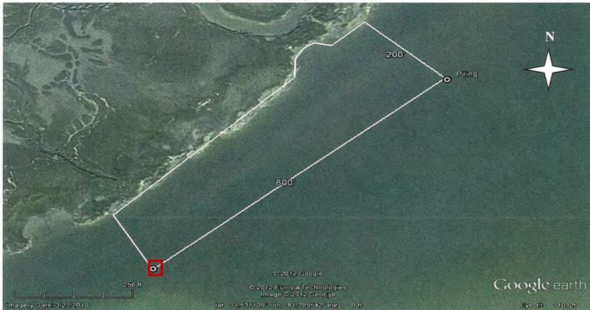
Figure 2. Reef Site Aerial Photograph shown with existing pilings, materials, and footprint (800' x 200'). For navigational purposes the southernmost piling is outlined in red
