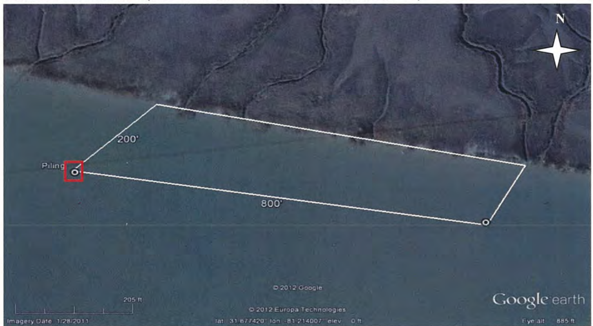
Figure 2. Reef Site Aerial Photograph shown with existing pilings, materials, and footprint (800' x 200'). For navigational purposes the southernmost piling is outlined in red.
