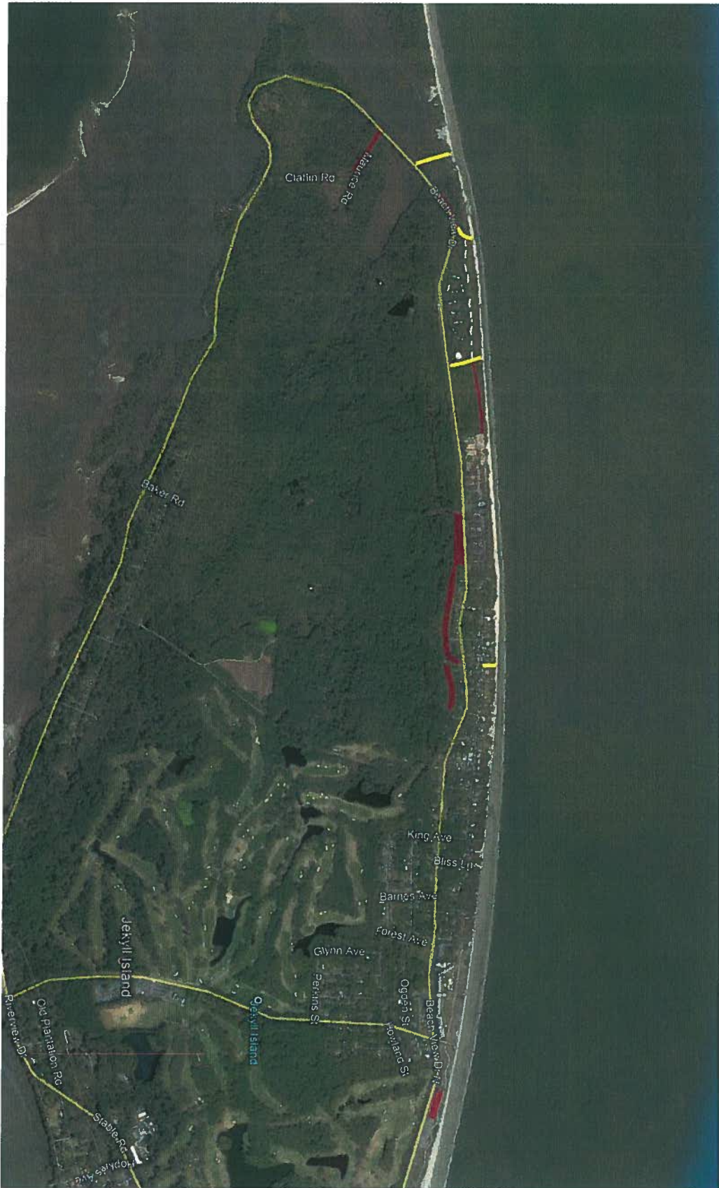
Figure 1. Prospective vehicle access routes (yellow) and material staging areas (red). From left (north) to right (south), the access routes are named, Driftwood Beach, Old North Picnic Area, Villas South, and Albright Lane. Of these. The only prospective staging area that falls within SPA jurisdiction is the southernmost one, on the right side of the image at Oceanview Beach Park, where there is an existing parking lot.
