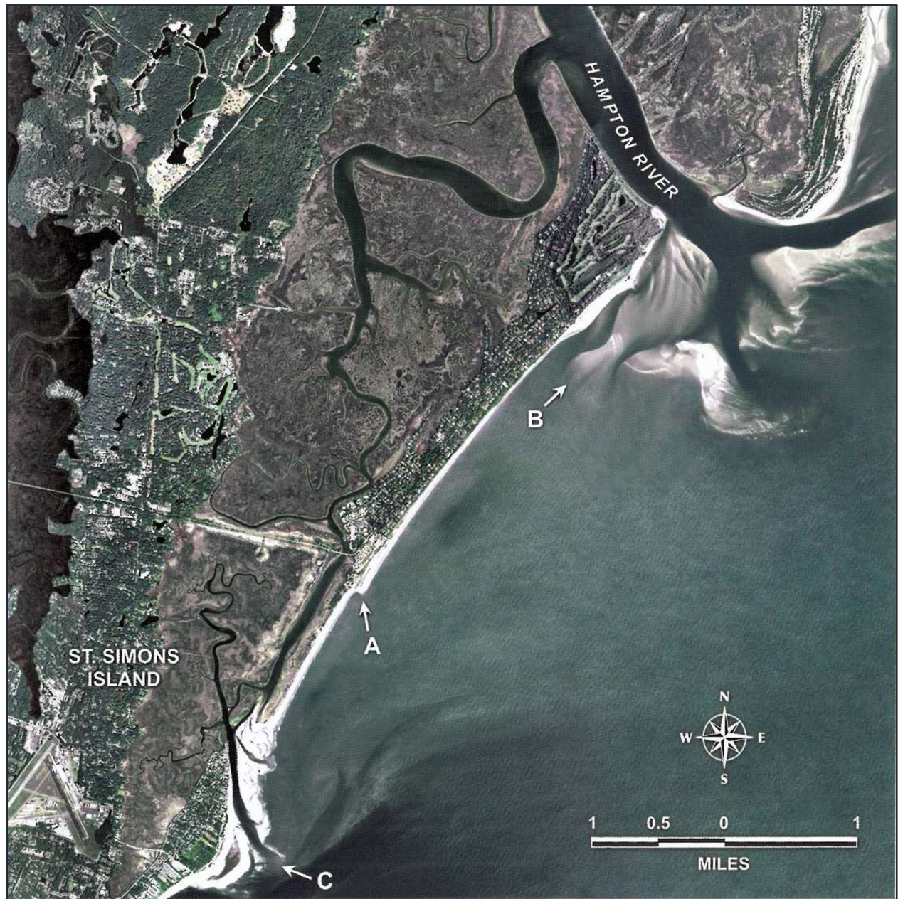
FIGURE 1.1. Vertical aerial image of Sea Island (GA) in 2009 showing extensive intertidal and subtidal shoals (ebb tidal deltas) of Hampton River Inlet and Goulds Inlet (“C”). “A” is the south groin/breakwater and “B” points to inshore shoals which influence the shape of the adjacent beach. [From Hayes & Michel 2013]
