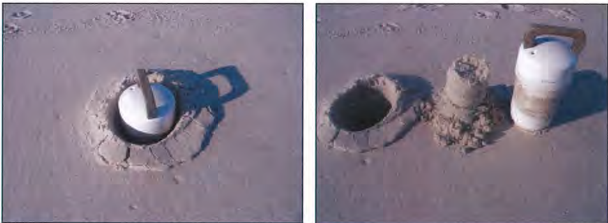
FIGURE 2.1. Uniform sediment samples were collected on the beach in the upper 6 inches (15 centimeters), mixed, and subsampled for laboratory testing.
