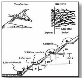
Figure 4.5.6b Installation of Brush Layering 1 Illustration Courtesy of: ianrpubs.unl.edu
