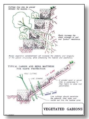
Figure 4.5.9e Installation of Vegetated Rock Gabions
