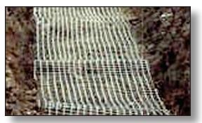
Figure 4.5.4b Geo-grid Photo Courtesy of: Pavingexpert.com
