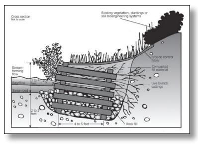
Figure 4.5.10b Installation of Vegetated Cribwalls Illustration Courtesy of: USDA
