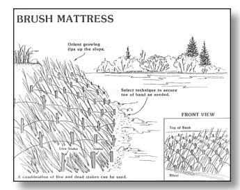
Figure 4.5.7b Installation of Brush Mattresses Illustration Courtesy of: Tara? Matt?
