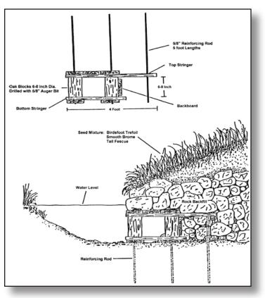
Figure 4.5.11g Installation of Fish Lunker Structure Photo Courtesy of: Vetrano, 1988 Chesapeakebay.net
