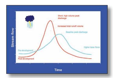
Figure 3.1c Hydrograph Representing Pre-and Postdevelopment Conditions Image Courtesy of: State.ga.us
