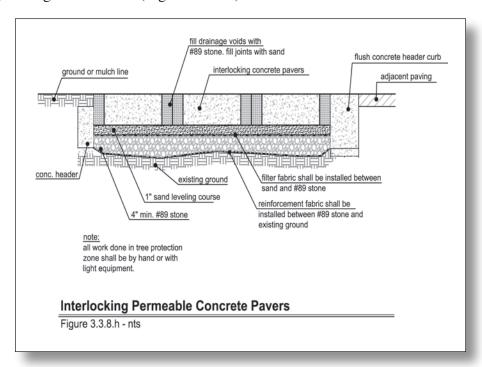
In addition to the relatively strict site constraints for porous pavement, a major limitation to the practice is the high failure rate some techniques have experienced in the field. According to EPA studies, 75% of porous pavement systems fail due to poor design, improper installation, use on soils with low permeability, traffic which exceeds the loading capacity and poor maintenance.
