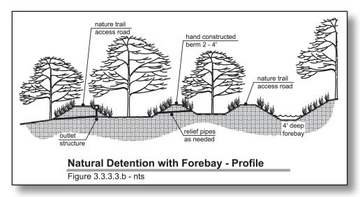
This is a practical, multi-functional solution for developments that must cross wetlands to access the buildable area of the tract. This practice creates a large green space area for the community, while detaining stormwater in the wetlands for infiltration and treatment by the soils and native vegetation. These natural detention areas can be installed with very little disturbance and require very little maintenance.
