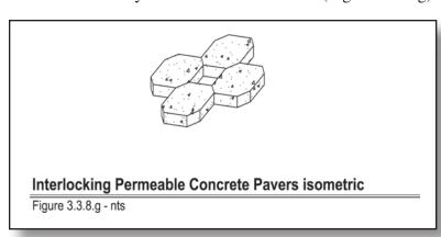
◆ Install permeable paving over the following base system unless its use is very light-duty and it is being installed on soils with infiltration rates exceeding 1 inch per hour. For unit pavers, the top 1-2 inches of the base is a layer of sand that also acts as a leveling course. Below that is a gravel base (porous concrete can be
