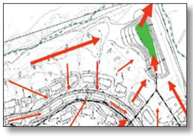
Figure 3.1b Decentralized Approach: Manage Stormwater at source with LID Techniques Image Courtesy of: PGDER
