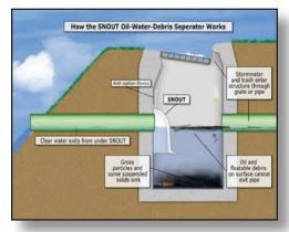
Figure 3.3.9c Illustration of a Snout Structure Image Courtesy of: Bestmp.com
