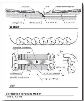
◆ During high flow events, inlets with overflow pipes are used to bypass the bioretention area and direct runoff to nearby collection and conveyance systems. The system may require using an additional infiltration or retention basin to pass runoff from larger storm events. Hand calculations and/or hydraulic/hydrologic modeling can determine the required storage volume. (Figure 3.3.4.f)
